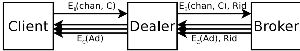
Figure 3: Message exchange for pub-sub ad dissemination. E_x(M) represents the encryption of message M under key x . B is the public key of the broker. C is a symmetric key generated by the client for only this subscription.
