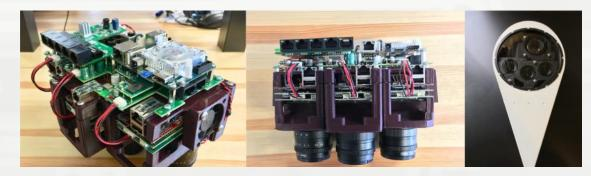
Mavrx adapted the AXIOM Beta by rotating and moving its sensor then removing one of the PCBs. This allowed them to fit three Betas, a DSLR and a Control and Image Storage Computer snuggly into their airborne camera pods. Ingenuity and collaboration helped them prototype a next-generation, multi-spectral camera system.
