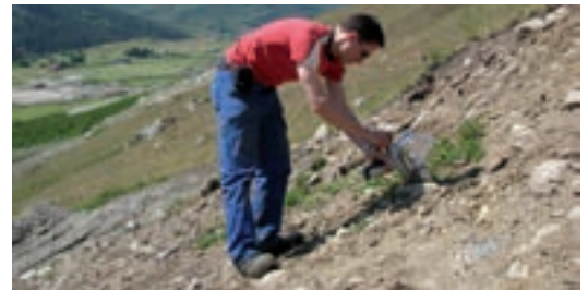
The lead content of a soil sample is determined using a mobile x ray fluorescence device
