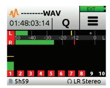
To effectively use NoiseAssist, start with the default setting of -6 dB and dial in more or less depending on your environment. An ideal setting will reduce the background noise without coloring the sound.
