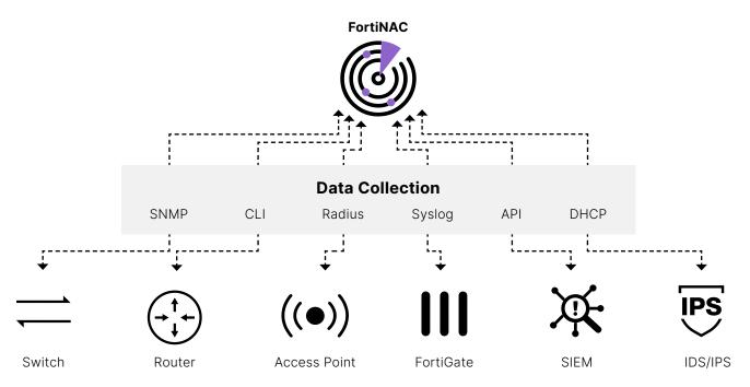
Figure 2: Supporting agentless data collection, FortiNAC provides extensive visibility into everything on the network.
