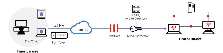
Figure 1: A typical Fortinet ZTNA user identity and access management implementation.
