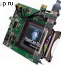
NetUP Dual DVB-S2-CI PCI-e Satellite Reception Card
