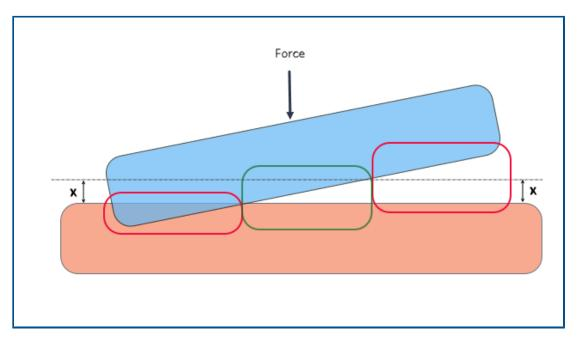
Contact detection is enhanced with a contact stabilization algorithm that can resolve under-constrained conditions. Contact stabilization acts as a numerical stabilizer by adding a small stiffness to qualified areas before they come into contact.
