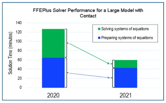
The solution time of linear static studies with many surface-to-suface contact elements is improved. The **Intel Direct Sparse** solver can handle linear static and nonlinear studies with more than 4 million equations.
