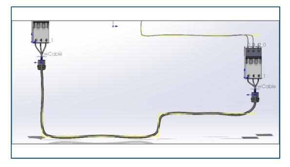
You can route electrical harnesses using splines.
