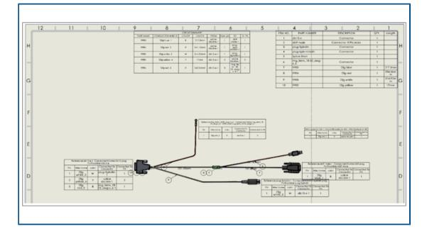
When you generate a flattened route, the tables are inserted in specific locations.
