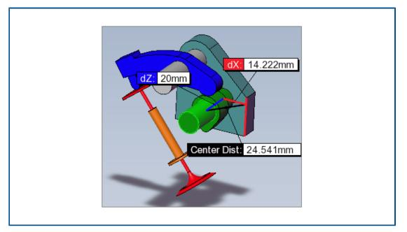
You can use the **Measure** tool to measure distances between planar-cylindrical and cylindrical-cylindrical faces. Different options specify the distance to measure when you select arcs or circles.
