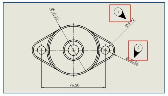
In drawings, you can tag inspection points according to VDA requirements. VDA balloons are frequently used in the German automotive industry.
