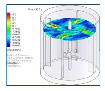
You can calculate free surface for models, including rotating equipment. This simulates fluid flow subjected to rotating systems as mixers for items such as consumer products, pharmaceuticals, and food.
