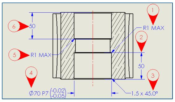
You can rotate VDA balloons while keeping the balloon number vertical. You can also adjust the font size for VDA balloons.
