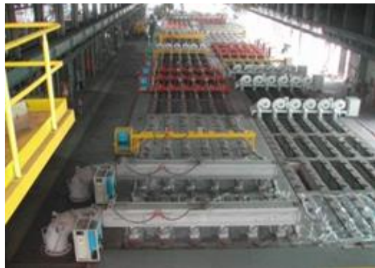
Anode baking furnace
