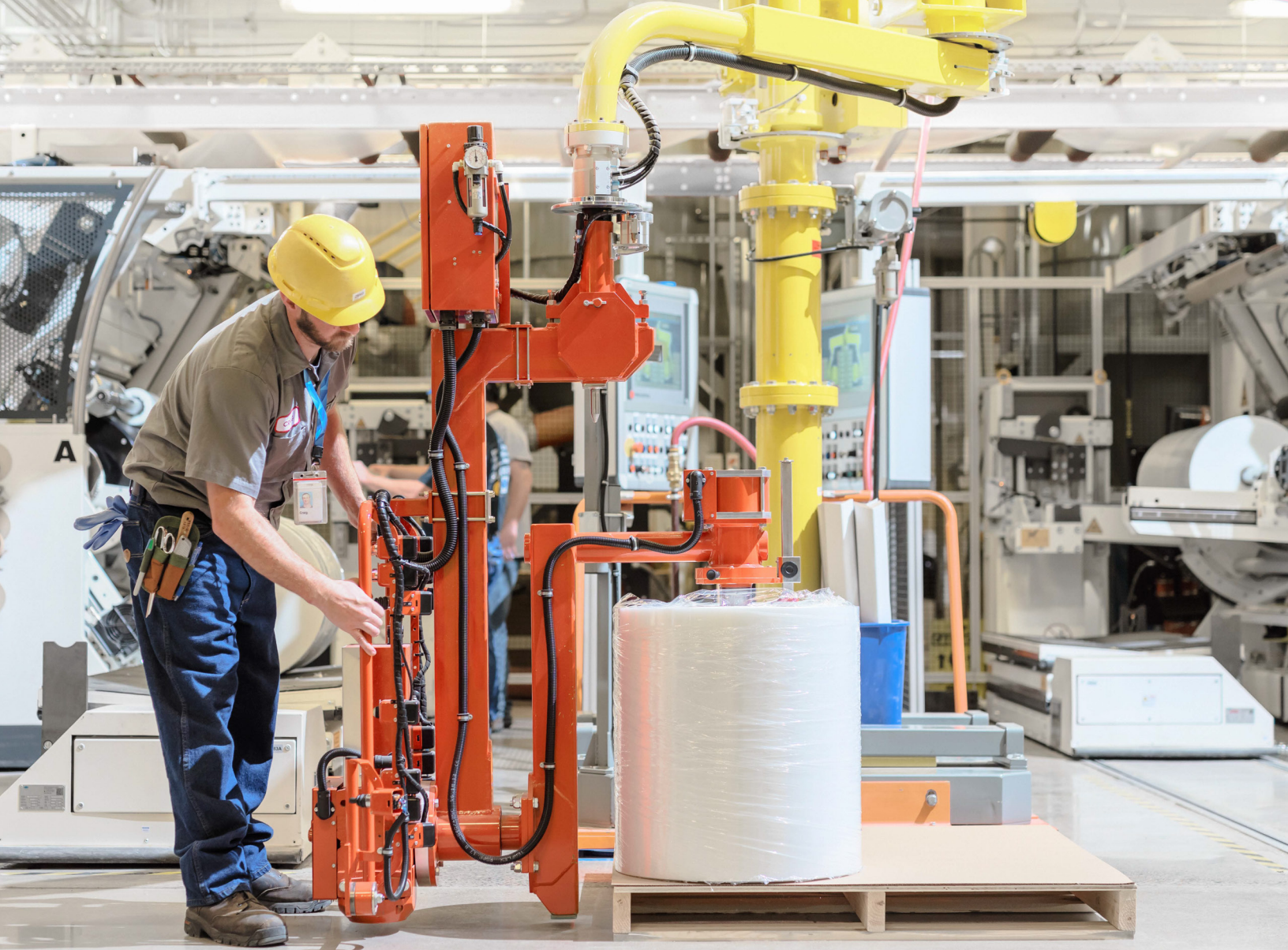
An operator uses a manipulator to safely place a roll of plastic onto a pallet.
