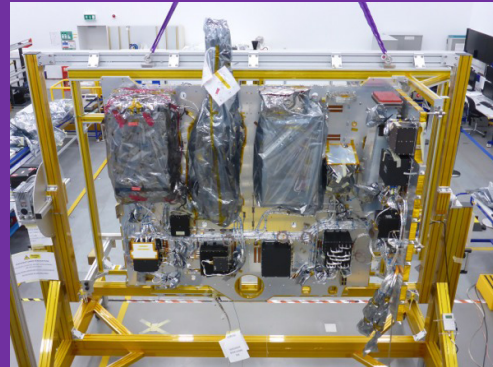
SO/PHI E-UNIT FM during the fly harness integration
