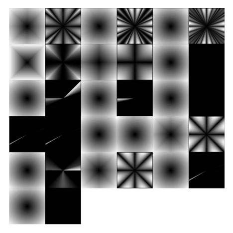
**Figure 4.** Results of various distance transform algorithms applied to an image consisting of 3 single-point objects. Top row, left to right: CDA 3x3, CDA 5x5, CDA 7x7. Second row, left to right: Chessboard, Cityblock, CSED. Third row, left to right: DRA 3x3, DRA 7x7, DV. Fourth row, left to right: 8SED, 8SED modified, Euclidean 3x3. Fifth row, left to right: 4SED, MD, MDDR. Sixth row: SimpleList.
