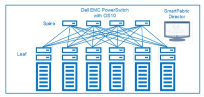
Data Center Network with bare-metal and VMware vSphere with BGP-EVPN overlay
