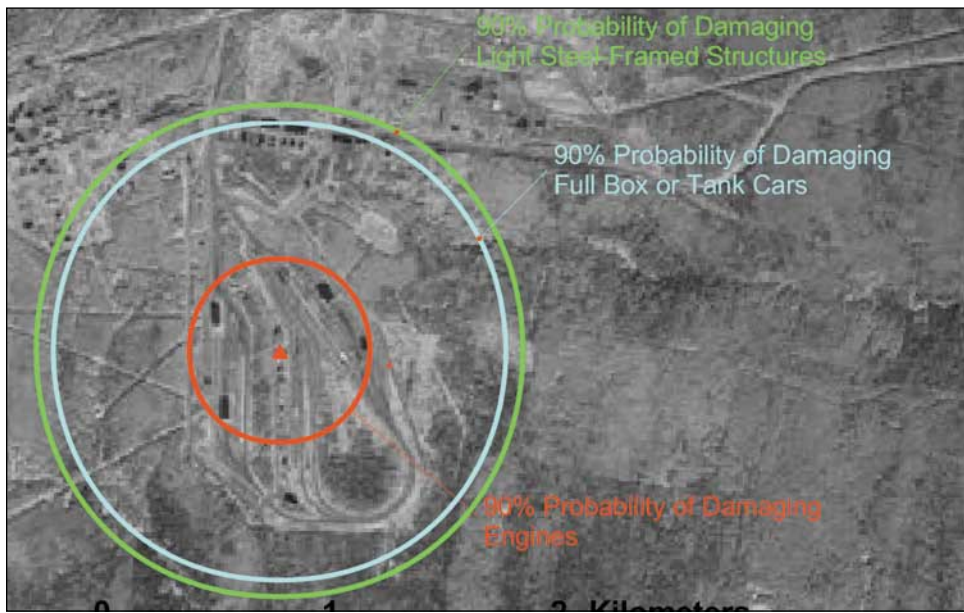
FIGURE 4.31 Damage Probability Contours for the Specified Target Types at the Bershet’ Rail-Mobile SS-24 Base
