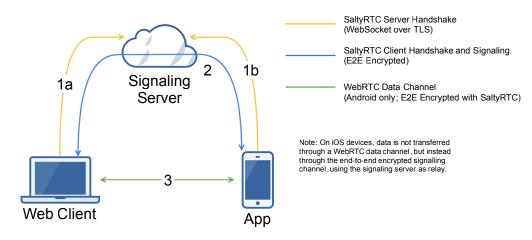
The web client and the app form a client-server relationship. All data about new events and old conversations is exchanged directly between the two through an end-to-end encrypted channel.
