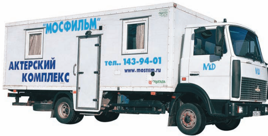
Trailer for actors mounted on the chassis of MAZ-4370
