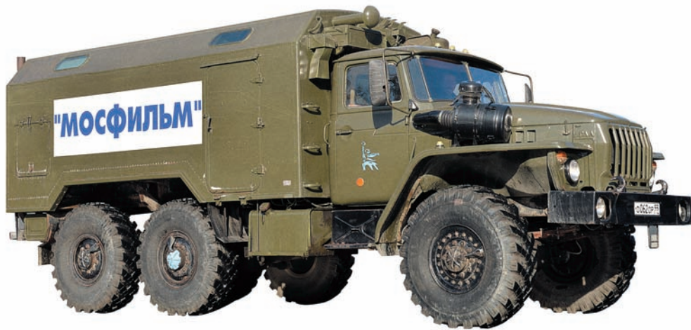
Mobile 100 kW power station (Lichtwagen) based on Ural 43203
