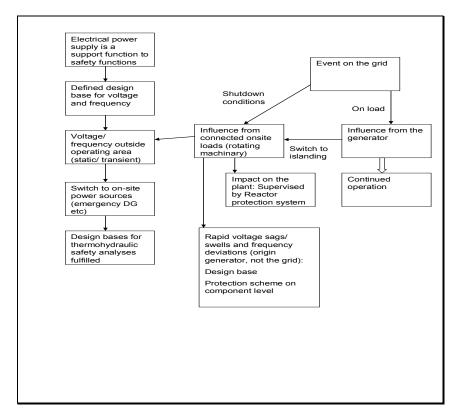
*Fig 4 Events originating from the grid. (Atmospheric disturbances not included).*
