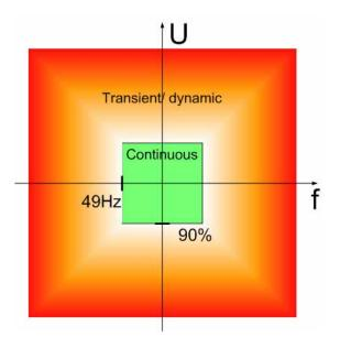
Fig 2 Operating area (example, levels to be omitted)
