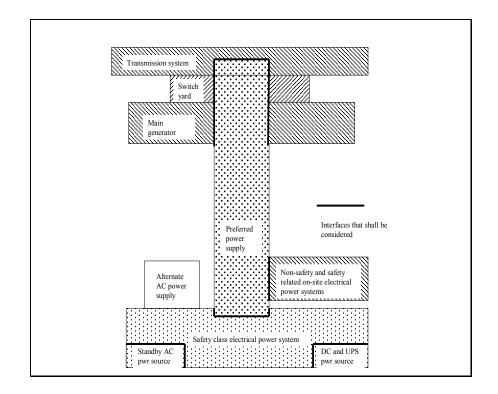
*Fig 3 Interfaces to be considered in the analyses (based on IAEA DS 430)*
