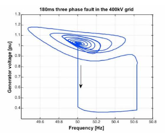
Example of on-site voltage (y-axis) and frequency (x-axis) variations during fault clearing on the transmission system
