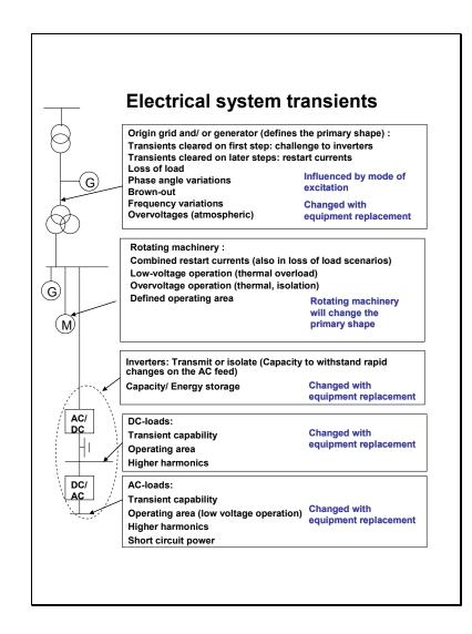
Fig 5 Electrical system transients originating from the grid
