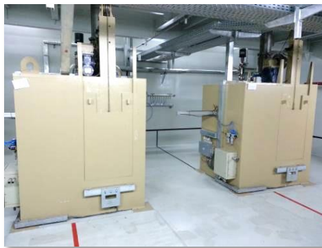
Figure 7.11. Camera for unloading of ash from the furnace of burning and camera of reburning
