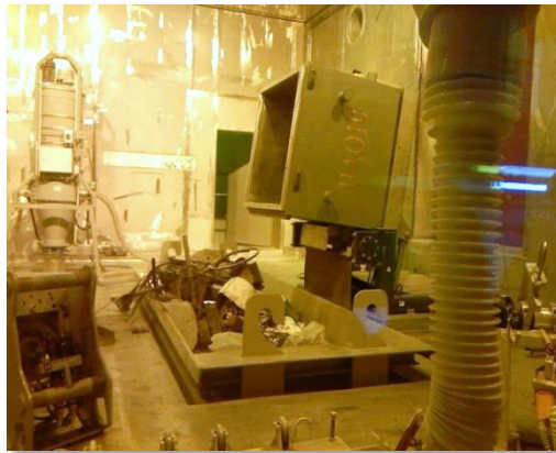
Figure 5.1. Emptying of skip into the receipt bay inside the SSR cell
