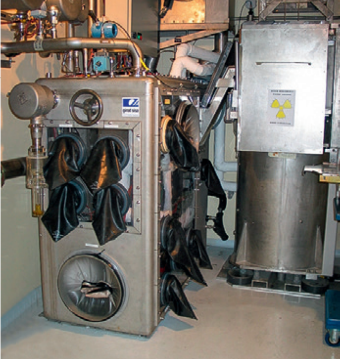
The EPICUR apparatus used for experiments on irradiating iodine species for the STEM project. IRSN, France
