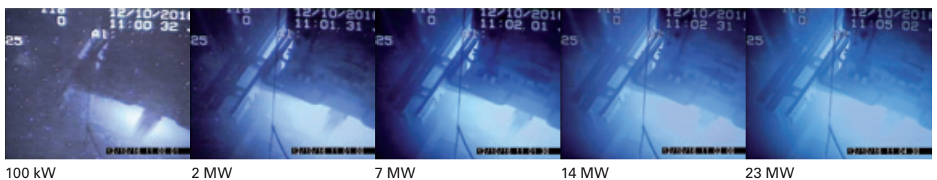
Figure 2: Photos looking down into the reactor pool showing the Cherenkov radiation characteristic of the different core powers
