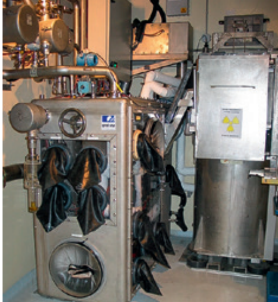
The EPICUR apparatus used for experiments on irradiating iodine species for the STEM project.
