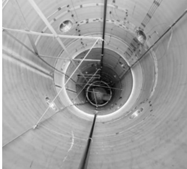
THAI test facility: top view into the open PAD vessel during instrumentation work.
