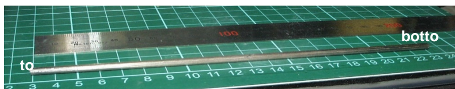
Figure 17.2. U-20 Pu-10 Zr fuel slug fabricated by injection casting method in a collaboration project between CRIEPI and JAEA
