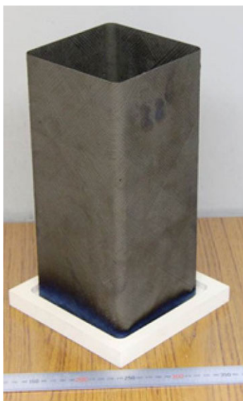
Figure 14.15. Appearance after the thermal shock tests by Toshiba
