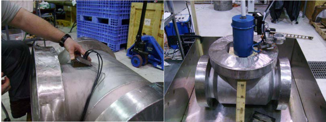
Figure 4: Photographs showing manual and automated inspection of the valve body in process
