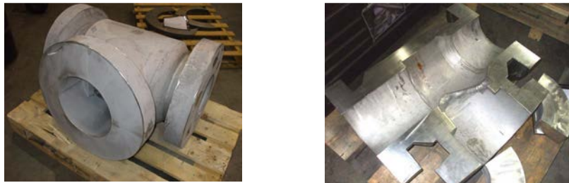
Figure 2: A 780kg (1716 lbs), 316L prototype stainless steel valve body produced during the feasibility assessment. The valve body was sectioned along its center line to reveal its ability to produce a sound, dimensionally stable, component configuration
