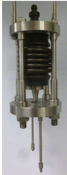
Figure 9: PLA test frame for segmented expanding mandrel
