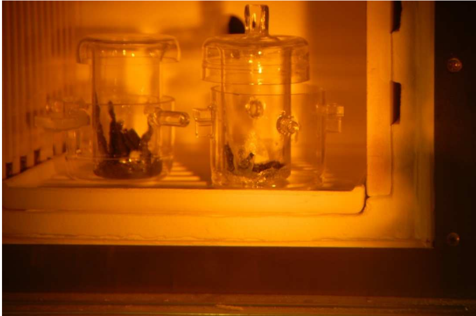
Figure 5: Graphite holder pieces following third burn step (96 hrs @ 900°C)
