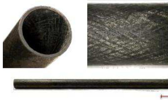
Figure 4: SiC Cladding with extra-fine machining
