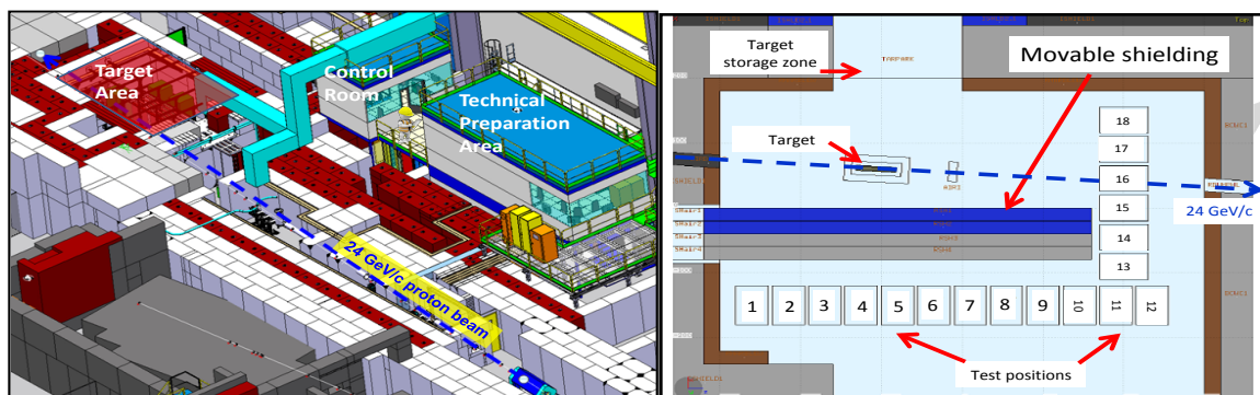
Figure 3: (a) Three-dimensional view of the facility and (b) FLUKA geometry for the target area
