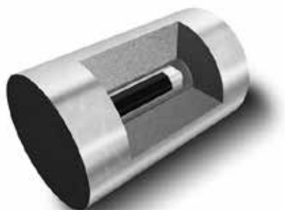
Figure 5: Artist's impression of OPERA supercontainer for heat-generating HLW
