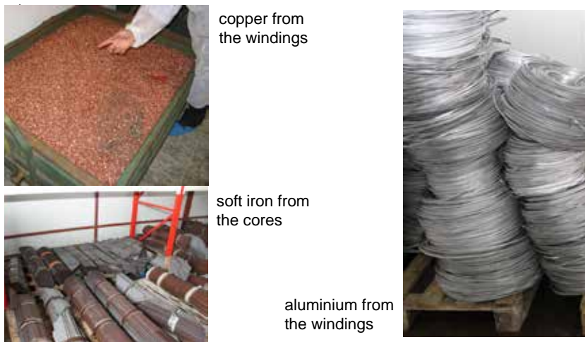
Figure 13: Products of cleaned transformers
