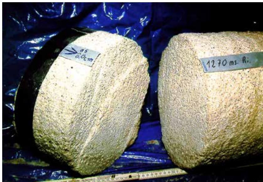
Figure 4: Final segments of a core drilled into old backfill from the 1 260/1 275 m floor of Riedel salt mine (Brenner, et al., 1999)
