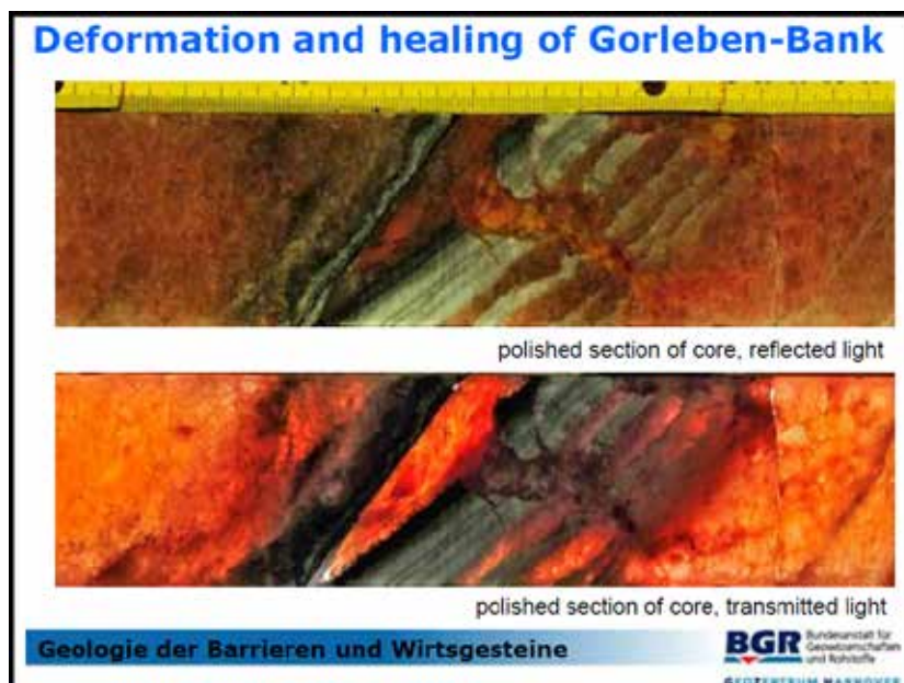
Figure 17: Deformation and healing of Gorleben-Bank
