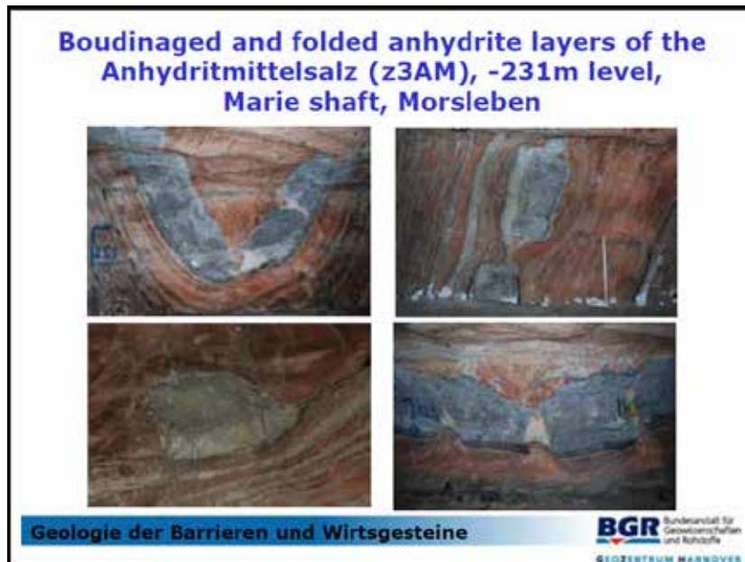
Figure 24: Boudinaged and folded anhydrite layers of the Anhydritmittelsalz (z3AM), -231 m level, Marie shaft, Morsleben
