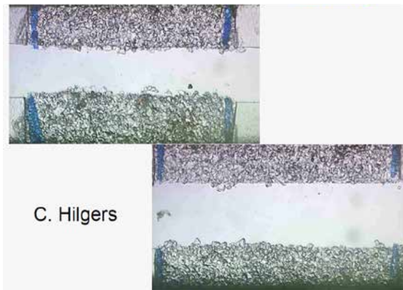
Figure 22: Experimental sealing of fractures in salts
