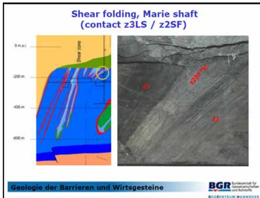
Figure 20: Shear folding, Marie shaft (contact z3LS/z2SF)
