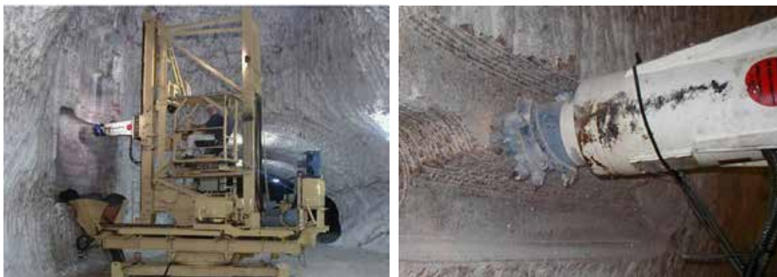
Figure 20: Cutting machine and cutter head
