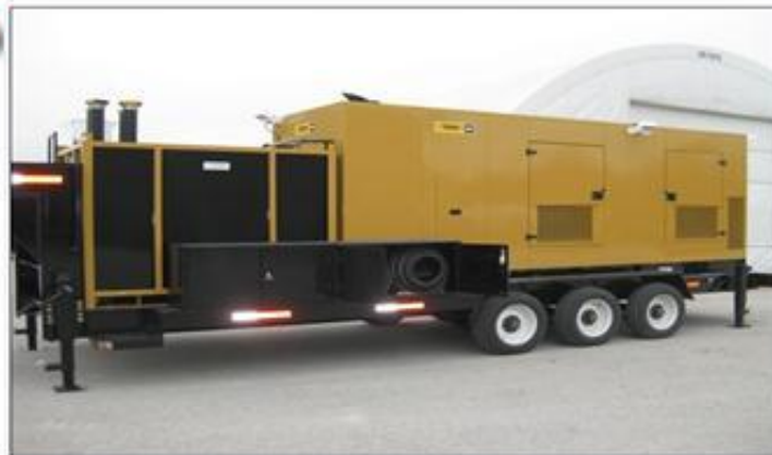
400 kW AC Generator
