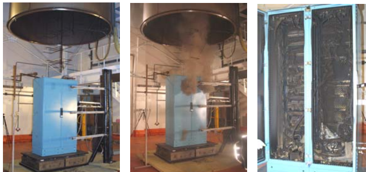
Figure 2. Fire test of real closed-door cabinet under large-scale calorimeter
