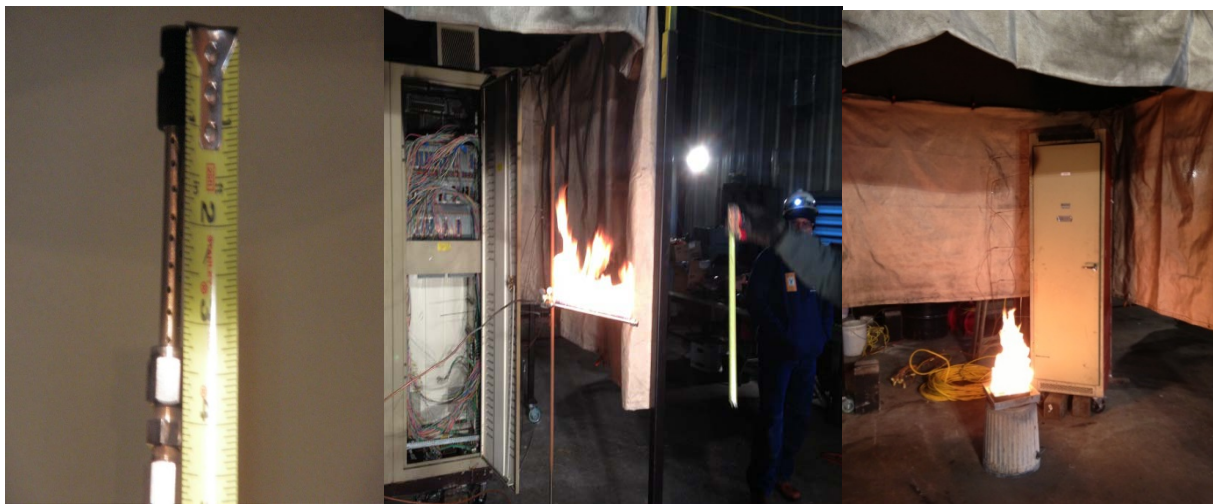
Figure 3. Ignition methods: 1-2kW propane burner (left), 10kW propane burner (middle), 20kW acetone pan (right)
