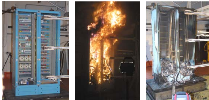
Figure 1. Fire test of real open-door cabinet under large-scale calorimeter
