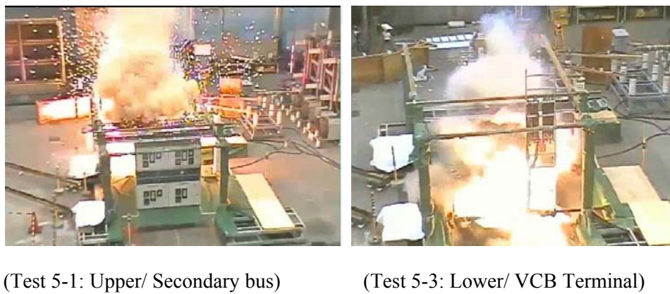
Figure 4. Test equipment layouts and test images for test series 5
