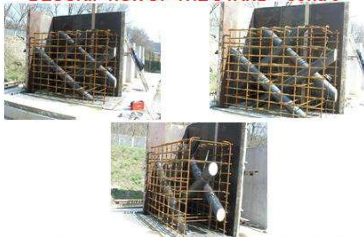
SPECIMEN No 5: CONTAINMENT WALL WITH REBARS AND DUCTS
