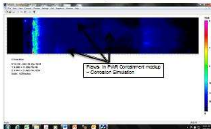
Flaws 1, 2 and 4 that were fabricated in the PWR Containment mockup
