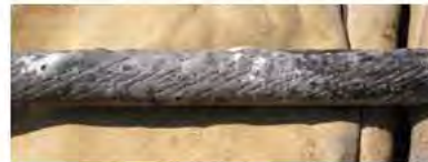
Gas leaking out of wireline.
