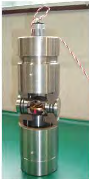
Inside picture of stress meter for horizontal and inclined components
