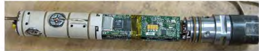
DS150: Seismometers on left with electronics in center and cable head connector on right.
