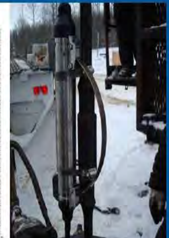
Deployment of a borehole geophone (ESG Ltd.)
