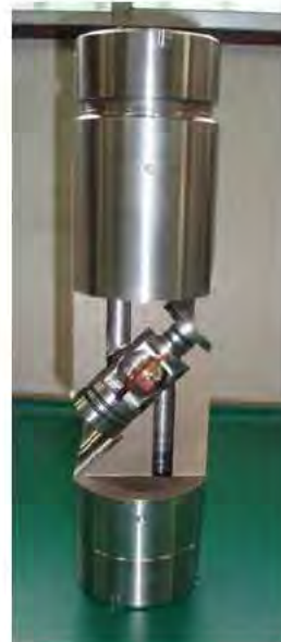
Inside picture of stress meter for horizontal and inclined components
