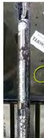
Top of Tiltmeter 1 after recovery from POD2
