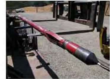
Tiltmeter POD before installation
