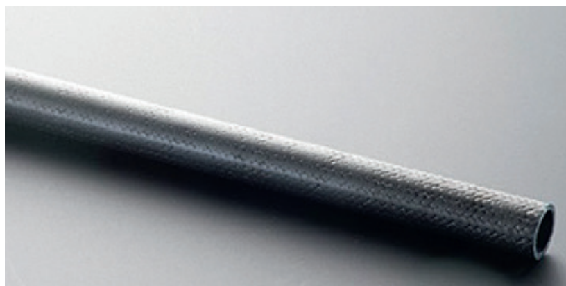
Segment of SiC/SiC fuel cladding including a metal liner.
