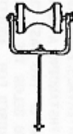
\frac{3}{8} " THRU-WALL BOLT APPROX. 10" LENGTH ONE WIRE RACK FOR BRICK OR FRAME CONSTRUCTION.
