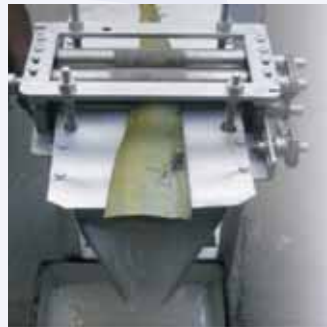
Aloe-vera Gel Extractor Capacity - 40-50 kg leaves/hr. Prototypes adopted: 10 units
