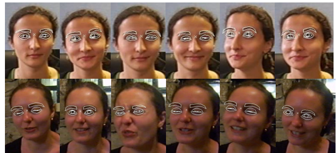
Fig. 11. Eye tracking in two example video sequences using our model, when blinking, face expression and small pose variations are involved.
