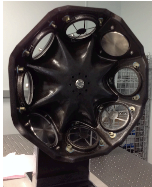
Figure 3-9: An early prototype of the element wheel. Pupil masks are shown on representative filters and the grism is represented by a mass model.
